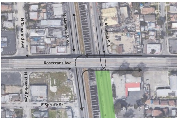
New vehicular circulation patterns enabled by extension of Rosecrans Avenue frontage roads. Bold arrows indicate key movements currently accommodated through Alameda East.
