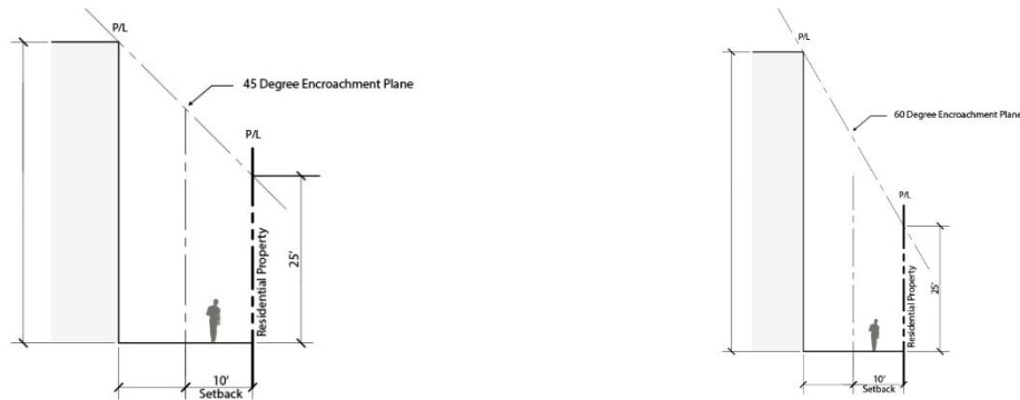
Required interior lot line height transition under base (left) and public benefit concession (right) standards.
